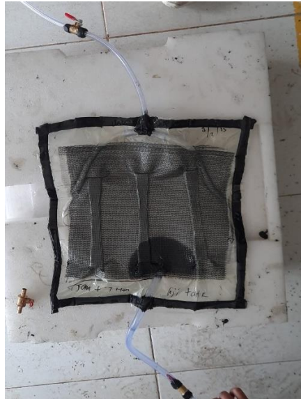
Gambar 3- 23 Proses Vacuum Infusion
