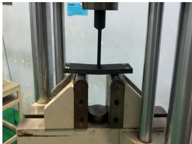
Gambar 4-1 Proses Pengujian Three Point Bending
