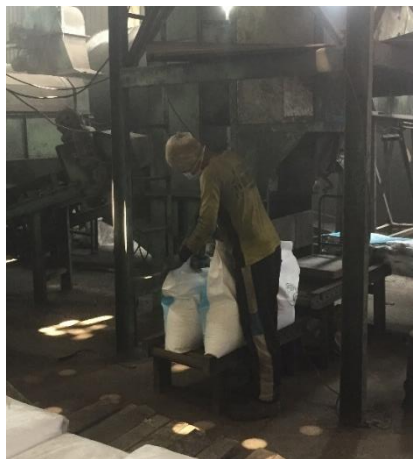
Gambar 4. 7 Proses Packing Pupuk
