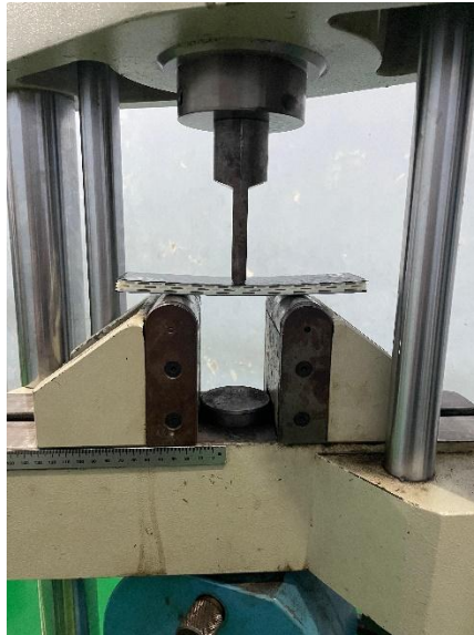
Gambar 3-29 Proses Pengujian Bending
