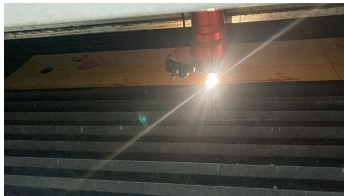
Gambar 4-4 Proses laser cutting cover mesin penggerak
