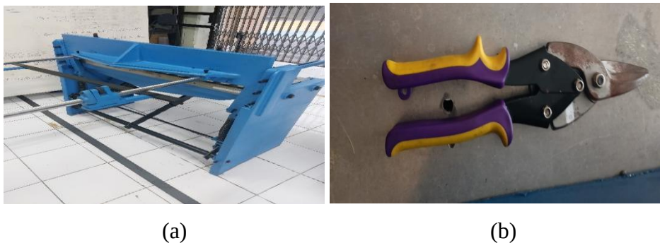
Gambar 3. 7 Alat potong plat (a) Mesin shear, (b) Gunting hollow
