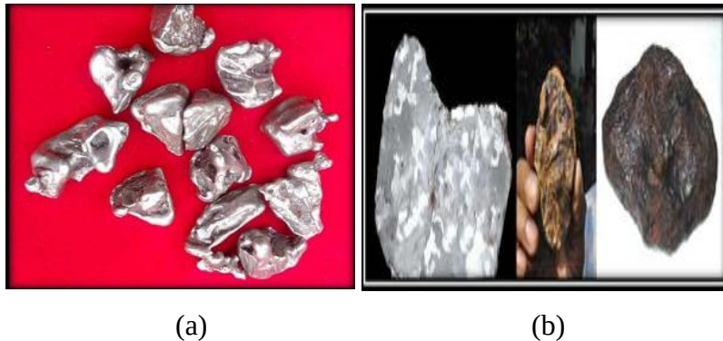
(a) (b) Gambar 2. 3 Material logam pamor (a) nikel, (b) batu meteorit (Sumber: (Adi, 2016))
