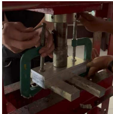
Gambar 3-13 Proses Compression Spesimen
