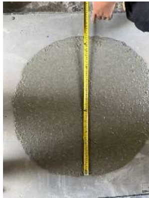
Gambar 1 Pengujian Slump Flow
