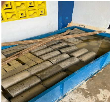
Gambar 1. Proses curing benda uji
