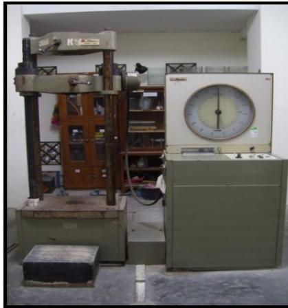
**Gambar 4.2 Mesin Uji Tarik Shimatsu Type UMH 30**
