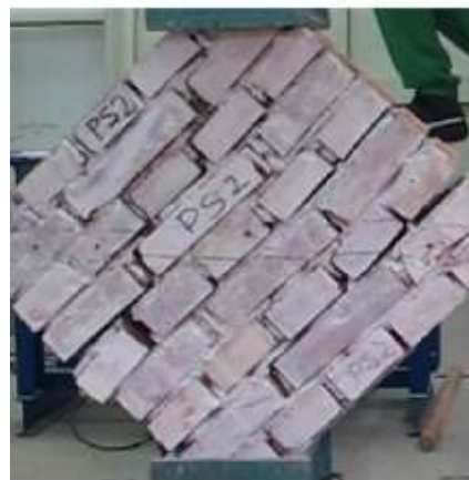
Gambar 1. Pengujian Diagonal Compression Test (Yardim & Lalaj, 2016)
