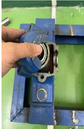
Gambar 3. 19 Pemasangan bearing ke bearing house
