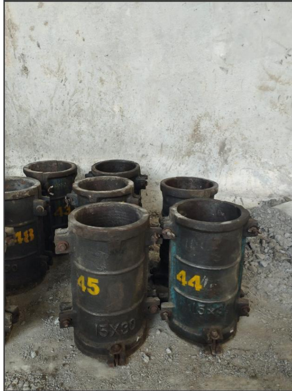
Gambar 7.3 Bekisting Siliner 15 X 30
