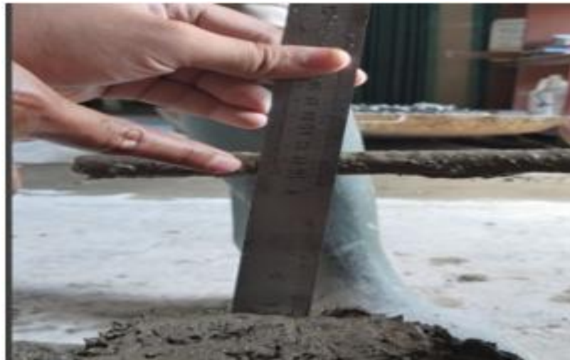
Gambar 6.2 Proses Uji Slump
