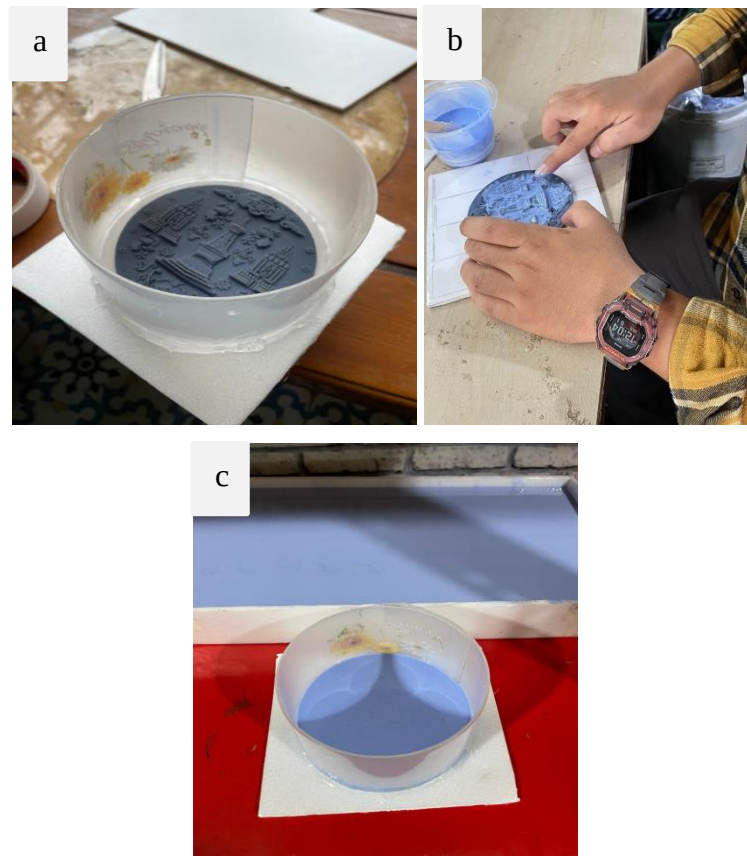
Gambar 3.5 Proses Penempelan Master (a), Proses Pengolesan Master (b), Proses Pengeringan (c)
