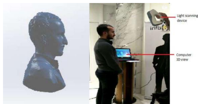
Gambar 2-2 Proses 3D Scanning (Sumber: Yalçinkaya et al., 2018)
