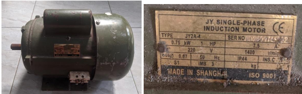
Gambar 3-21 motor listrik 1 HP 220 V 750 Watt 50 Hz
