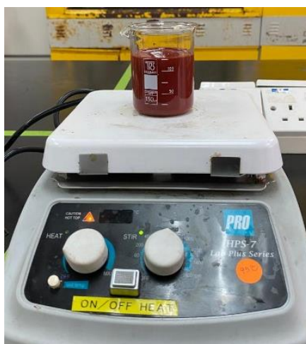
Figure 5.3.2.1 Lipstick ingredients being stirred using a magnetic stirrer.
