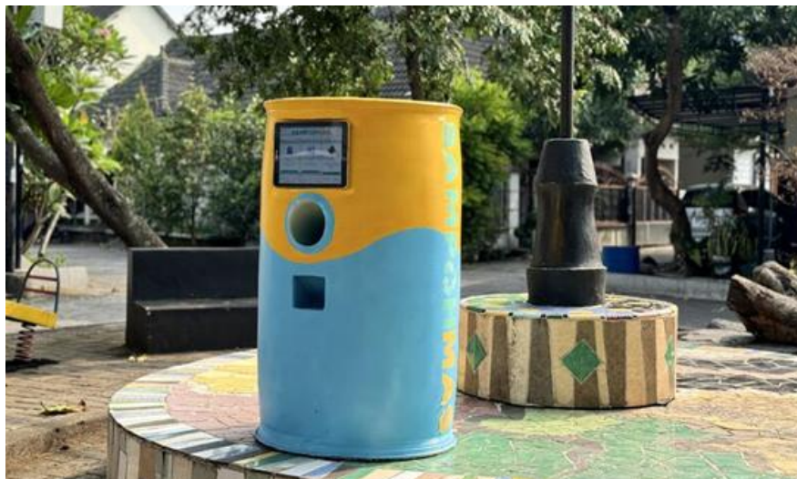
Gambar 4.26 Purwarupa Alpha Reverse Vending Machine
