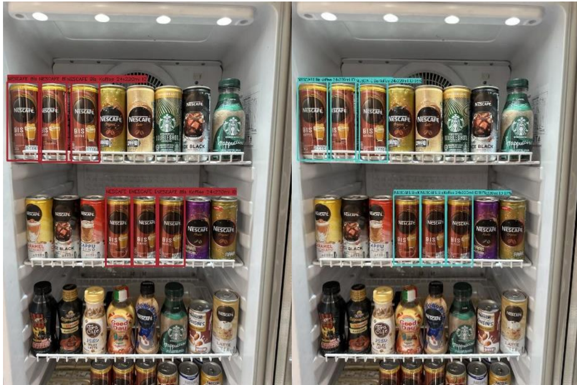
Gambar 4. 16 Kiri: Ground Truth. Kanan: Hasil Inferensi Model 320x320
