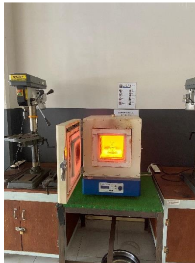
Gambar 3- 9 Proses Pack Chromizing
