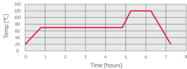
Gambar 2- 2 Multi-stage temperature cycle
