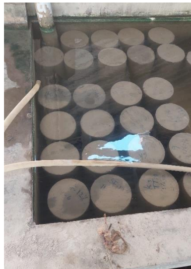
Gambar 5.8 Curing Benda Uji
