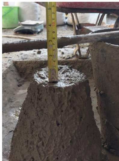
Gambar 5.7 Hasil Slump Test
