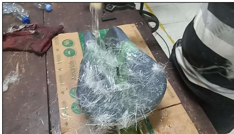
Gambar 4- 39 Perataan Serabut Fiberglass
