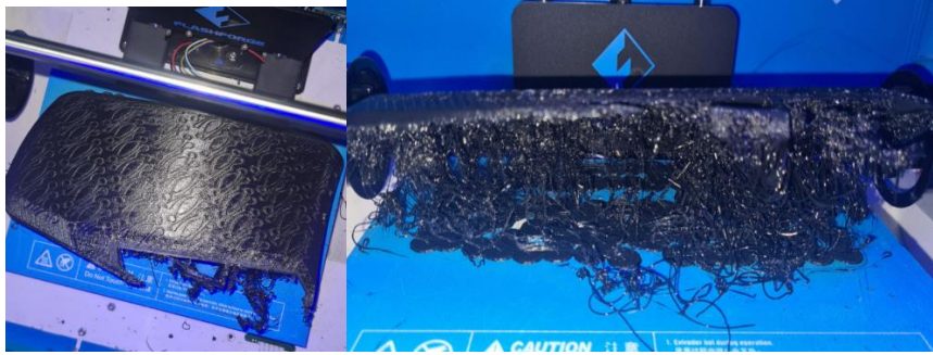
Gambar 4. 22 Proses 3D print percobaan 2
