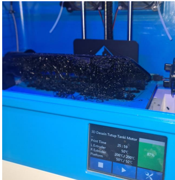
Gambar 4. 23 Percobaan 3D print gagal
