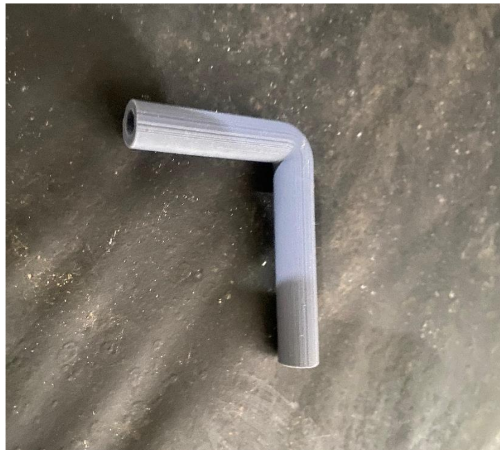
Gambar 4-38 Hasil 3Dprinting L Penerus Gaya Nozzle Cat Semprot Rubber
