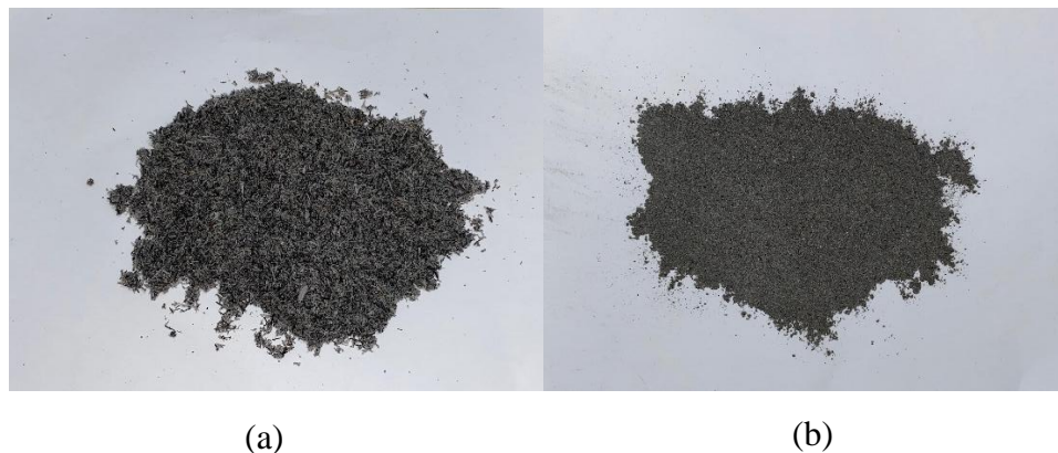
Gambar 3.1 (a) Abu Sekam Padi ( Rice Husk Ash ) dan (b) Abu Jerami Gandum ( Wheat Straw Ash )
