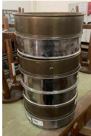
Gambar 4.5 Set Saringan Agregat
