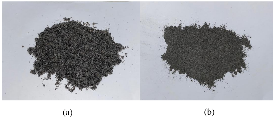
Gambar 4.4 (a) Abu Sekam Padi ( Rice Husk Ash ) dan (b) Abu Jerami Gandum ( Wheat Straw Ash )
