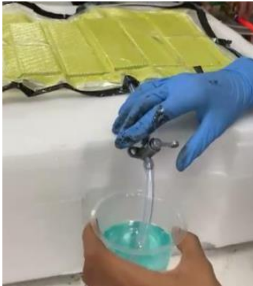
Gambar 3.31 Proses Vacuum Infusion
