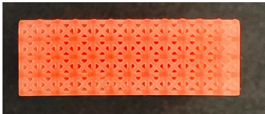
Gambar 3-33 Spesimen Core Density 60%
