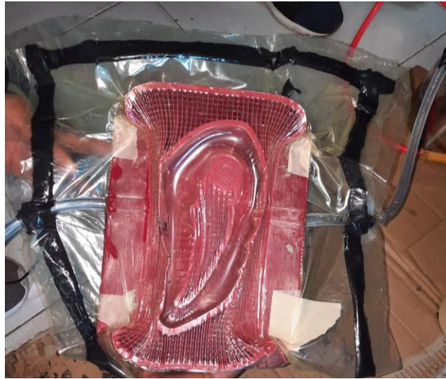
Gambar 4-7 Kondisi molding saat proses vacuum
