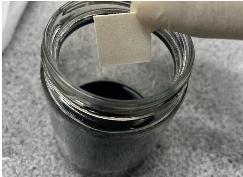
Figure 3.3: Coating for specimen membrane
