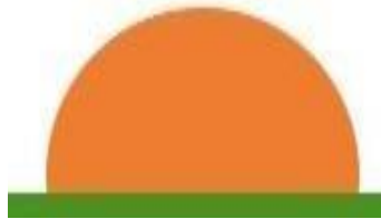
Figure 2.7: Oleophobic contact angle
