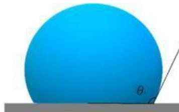
Figure 2.5: Hydrophobic contact angle
