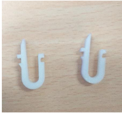
Gambar 4. 27 Hasil 3D Printing Snap Fits
