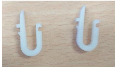
Gambar 4. 17 Hasil 3D Printing Snap fits
