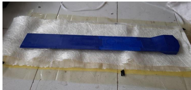
Gambar 3.20 Persiapan vacuum infusion
