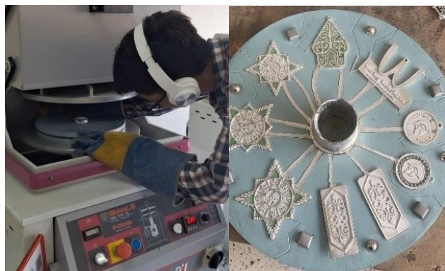
Gambar 3- 32 Proses Pasca Pengecoran Spin Casting
