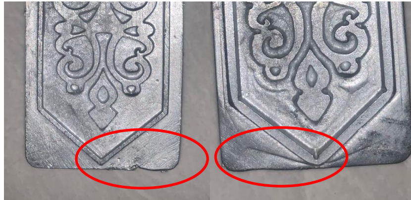
Gambar 4. 28 Hasil spin casting CCW 700 rpm percobaan 1
