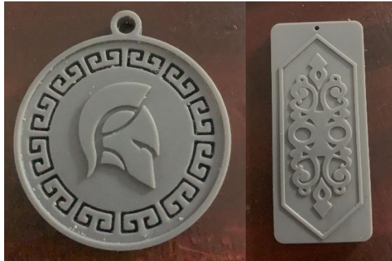
Gambar 4. 3 Master produk 3D print resin
