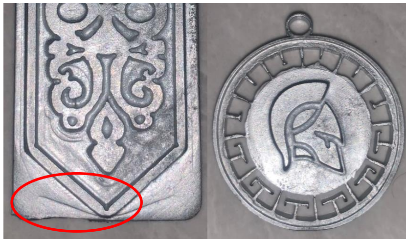
Gambar 4. 29 Hasil spin casting CCW 800 rpm percobaan 3
