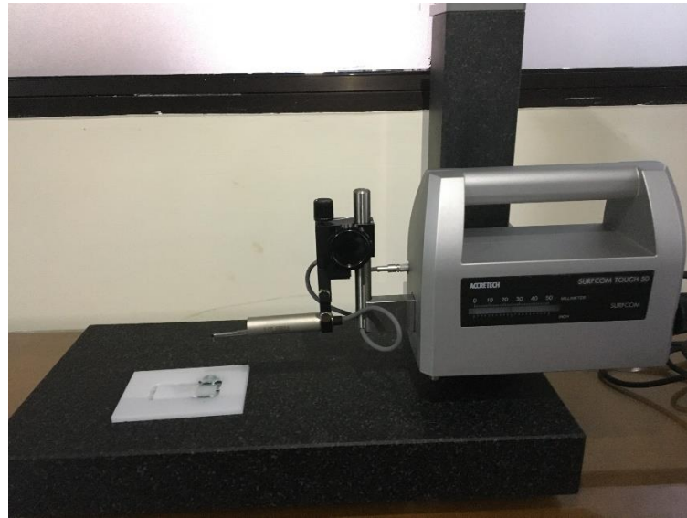
Gambar 3-11 Alat Ukur Surfcom Touch 50
