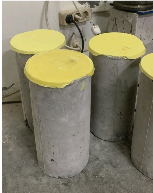
Gambar L.3.3 Proses Caping Benda Uji
