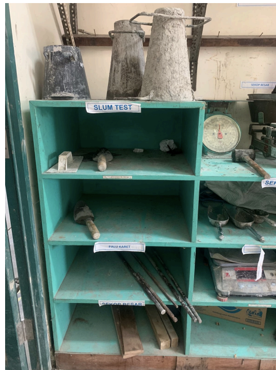
Gambar L.1.1 Peralatan Mixing Beton
