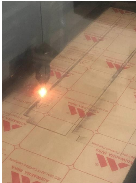
Gambar 4.5.2-1 Proses Laser Cutting Akrilik
