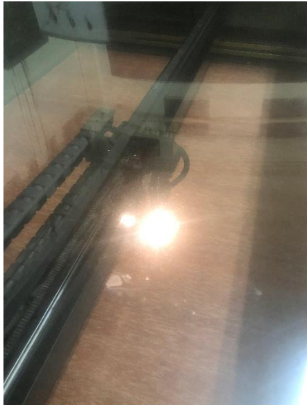
Gambar 4.5.2-2 Proses Laser Cutting Triplek
