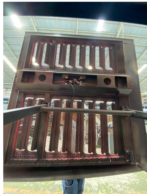
Gambar 4. 25 Bagasi Flap Radiator (Dalam) Legacy SR 3 XHD Prime Ultimate Series Sumber: PT. Laksana Bus Manufaktur
