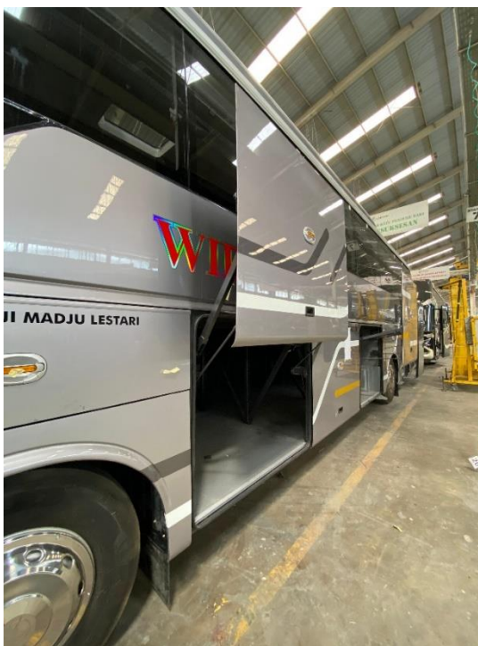
Gambar 4. 26 Bagasi (Luar) Legacy SR 3 XHD Prime Ultimate Series Sumber: PT. Laksana Bus Manufaktur
