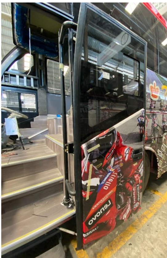
Gambar 4. 14 Pintu Depan (Luar) Legacy SR 3 XHD Prime Ultimate Series Model Sliding Door
