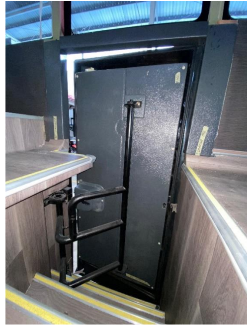
Gambar 4. 17 Pintu Belakang (Dalam) Legacy SR 3 XHD Prime Ultimate Series Model Sliding Door Sumber: PT. Laksana Bus Manufaktur
