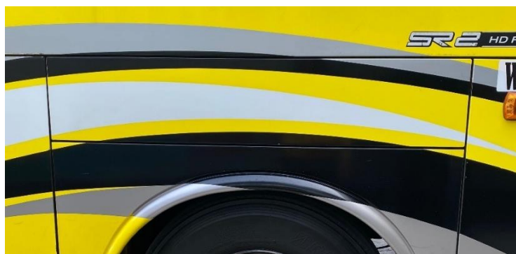
Gambar 4. 12 Lambung Mati Legacy SR 3 / SR 2 HD Prime Sumber: PT. Laksana Bus Manufaktur
