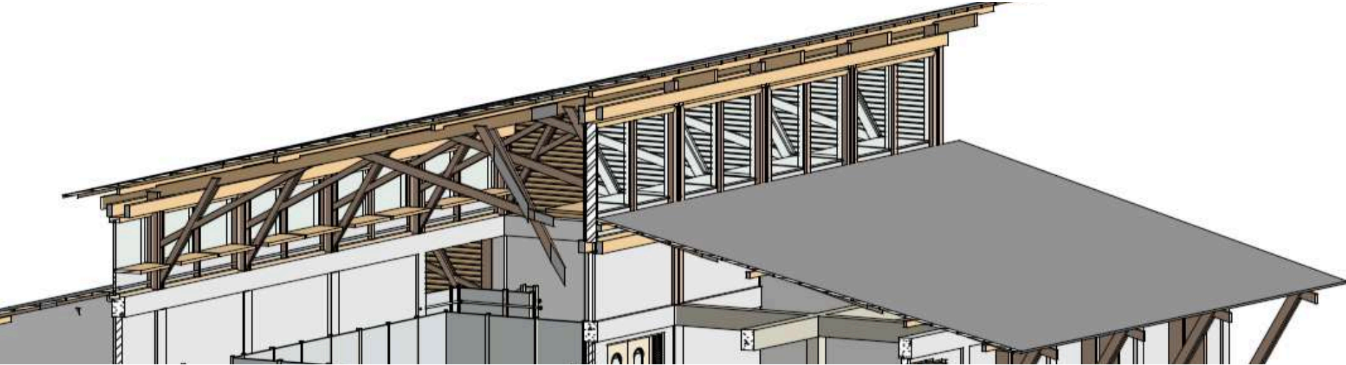
Figure 4.14 The detail of clerestory windows and the light shelves Source: Author, 2024
