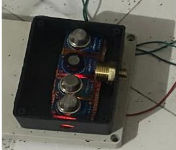
Gambar 4.3 Rangkaian Sensor Gas
