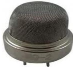
Gambar 2.1 Sensor gas MQ-2
