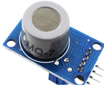
Gambar 2.3 Sensor Gas MQ-7
