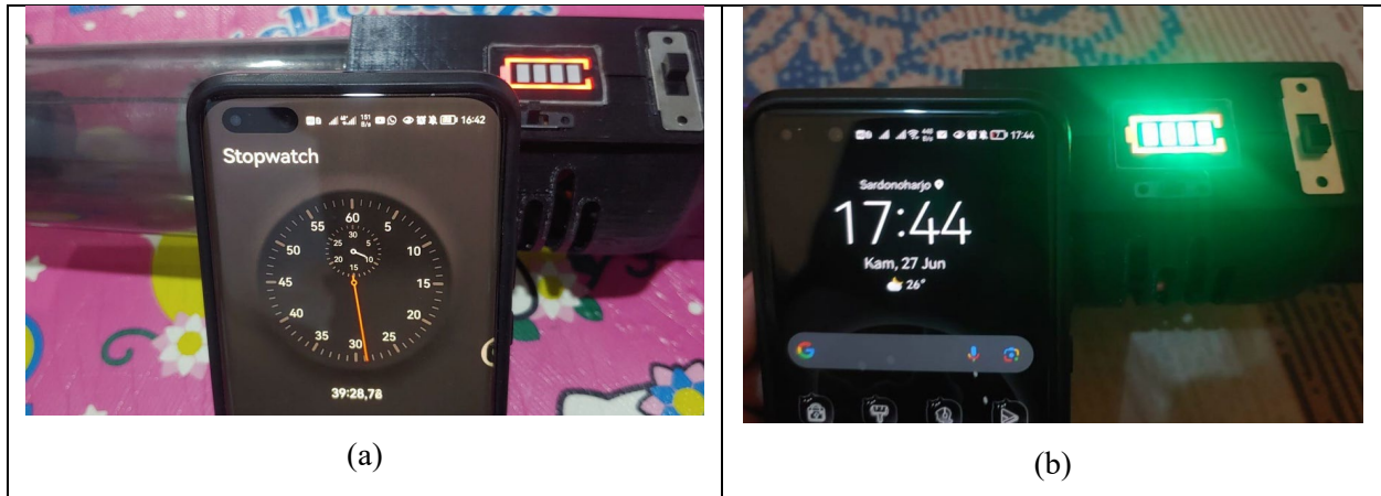
Gambar 5.11 (a) Mulai pengisian vacuum , (b) Selesai pengisian vacuum
