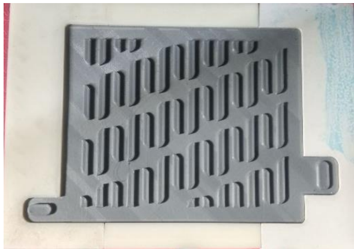
Gambar 4-28 Hasil 3D print molding revisi
