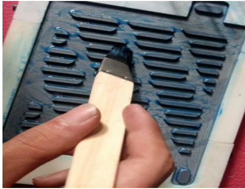
Gambar 4-29 Pelapisan cairan release agent PVA
