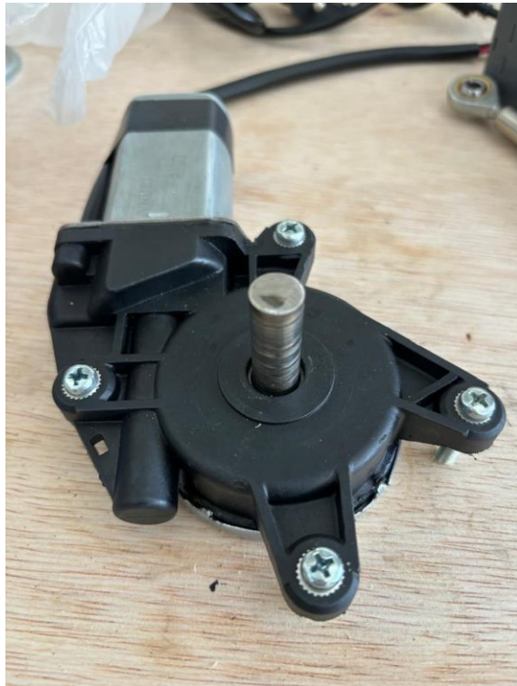
Gambar 4- 10 Motor Sesudah Dipasangkan Stainless Steel
