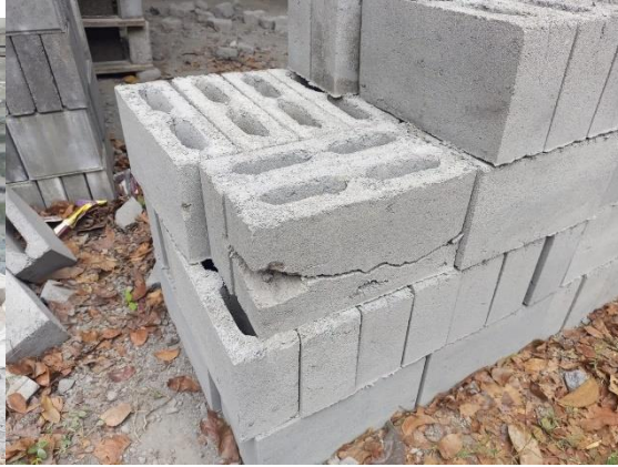
Attachment 20: Failed concrete brick
