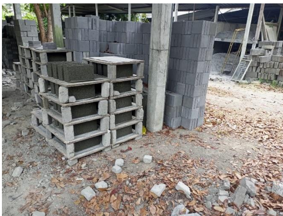
Attachment 35: Drying concrete brick
