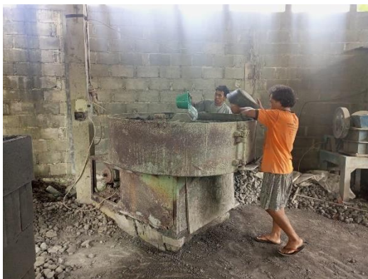
Attachment 11: The worker is pouring sand into mix machine Attachment 12: The mix machine is mixing
