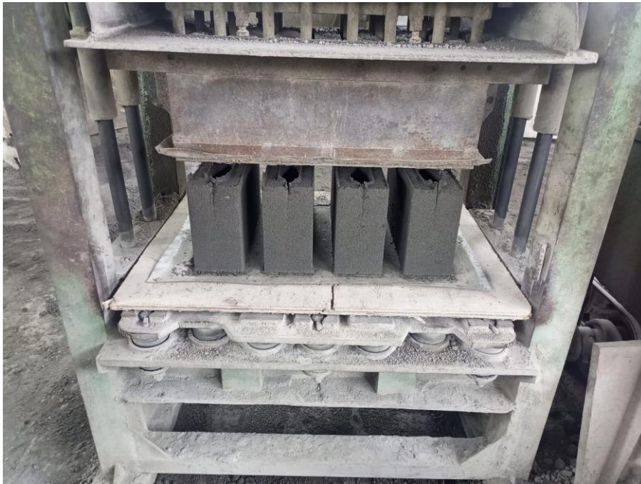
Figure 4.5: Concrete brick after being pressed
