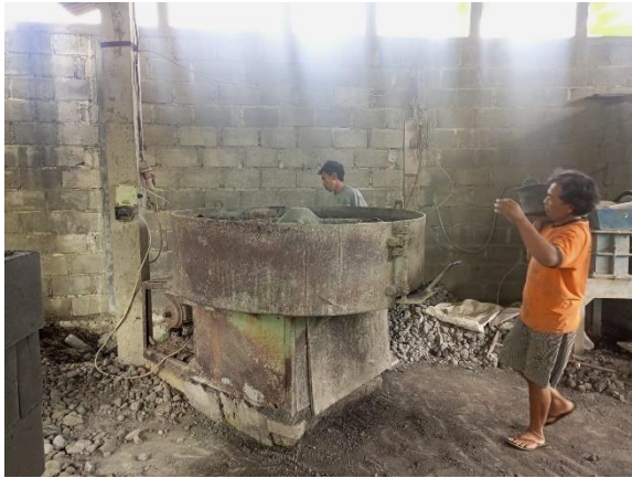
Attachment 1: Worker delivering sand into mixer
