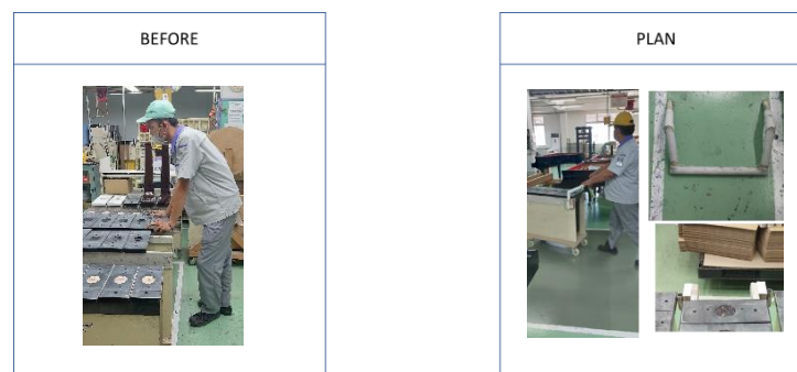
Gambar 4. 11 Rancangan Handling Rak Leg Piano
