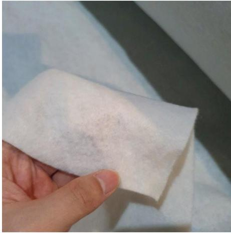
Gambar 3- 10 *Breathe Bleeder Fabric*
