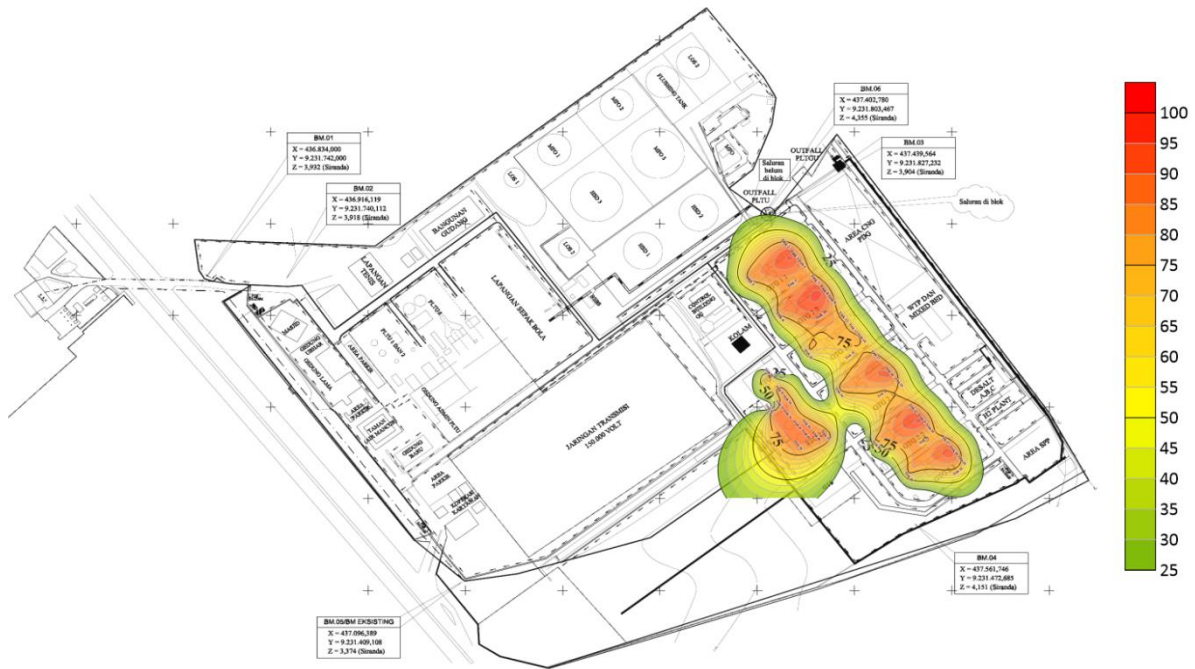
Gambar 4.18 Noise Mapping GTG (Gas Turbine Generator) dan STG (Steam Turbin Generator)
