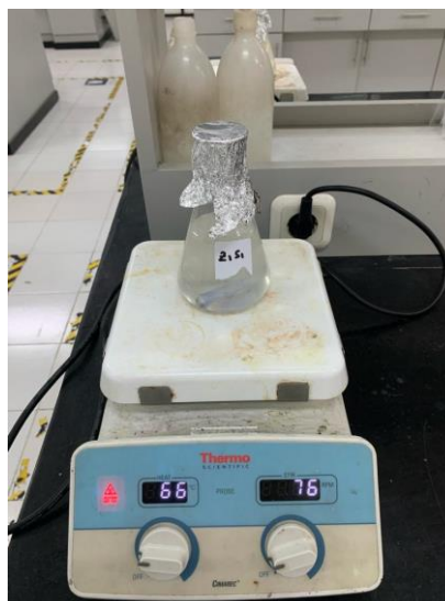
Gambar 3. 7 Proses WPO Sampel Mikroplastik
