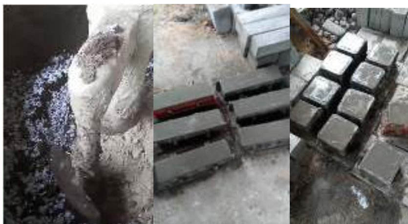
Figure 5.2 Mixing and pouring process of papercrete
