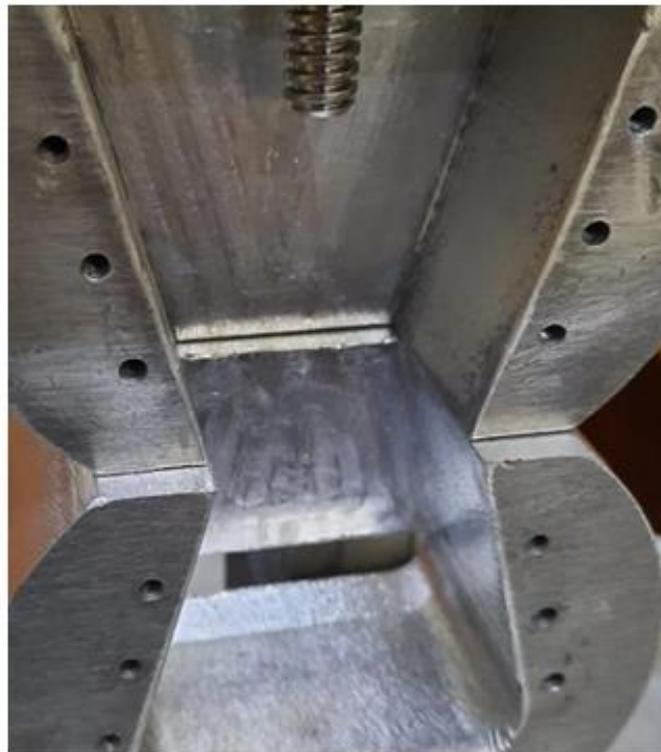
**Gambar 3- 3 Misalignment gripper**
